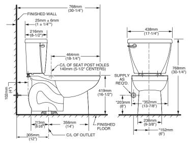
NOTES: THIS TOILET IS DESIGNED TO ROUGH-IN AT A MINIMUM DIMENSION OF 305MM (12") FROM FINISHED WALL TO C/L OF OUTLET. SUPPLY NOT INCLUDED WITH FIXTURE AND MUST BE ORDERED SEPARATELY
