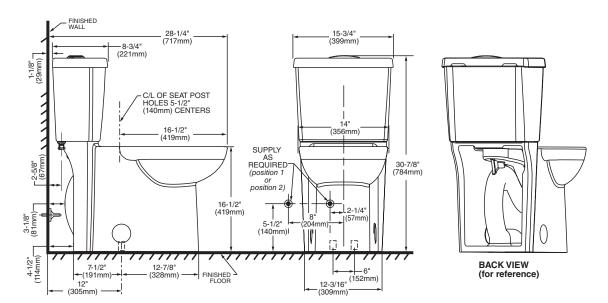
IMPORTANT: Water supply on the wall is required at 2-1/4" or 8" from centerline of the toilet (see rough-in). First suggested position is hidden behind the toilet. The geometry of the toilet gives space for this installation. The second suggested position is next to the toilet. Between these two positions, the space for the supply between wall and toilet is limited to 4-1/2". In this case, check your supply and hose dimensions.
