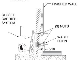
Using a level, adjust the top left back-up nut so that it is in the same vertical plane as the lower left back-up nut. (If wall surface is irregular, the three back-up nuts must be positioned to allow a minimum 1/16" gap between fixture and wall surface.)
