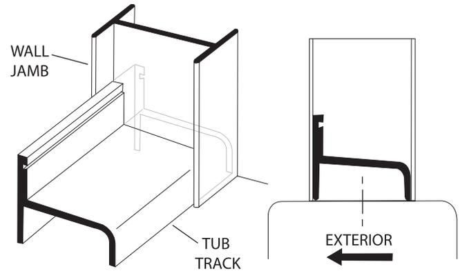
**2** Use a level to plumb both wall jambs [B], then mark the pre-drilled hole locations on the wall. Lightly mark along both sides of the tub track [A] with a pencil, then remove all parts.
