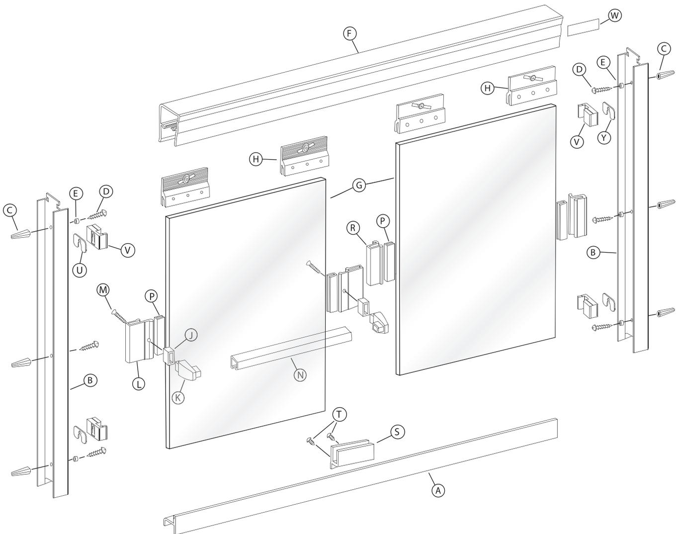
**1** Measure the wall-to-wall opening at the center of the tub rim. Cut the tub track [A] 1/16" short of this dimension. An inexpensive miter box available at your local hardware store will help you get clean square cuts.
