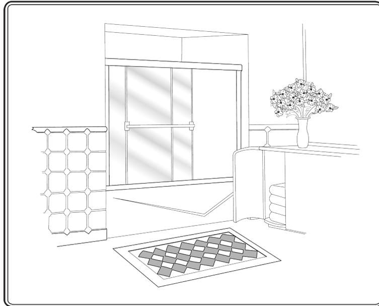
**MAINTENANCE:** Two primary materials are used to manufacture your new Aquatic enclosure: tempered glass and anodized aluminum. To assure a long lasting finish on the enclosure, wipe it down with a towel after each use. Never use a scouring agent to clean the aluminum.
