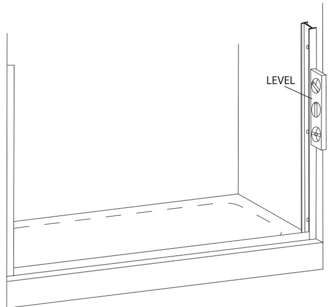
**3** Before replacing the tub track [A], force a slight downward bow in the extrusion. This will ensure the track fits tight to the tub. Run two beads of caulk inside the penciled marks on the tub rim. Place the tub track in the exact position marked in Step #2 and seat it firmly in the caulking.
