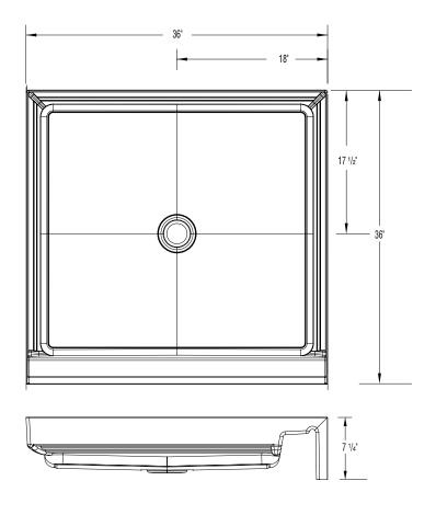
FEATURES | Ibs (kg) Dimensional Tolerance ± %". Dimensions needed for site preparation should be measured from the unit. Aquatic assumes no responsibility for preparatory work.
