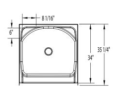
FEATURES | Ibs (kg) Dimensional Tolerance ± 36". Dimensions needed for site preparation should be measured from the unit. Aquatic assumes no responsibility for preparatory work.
