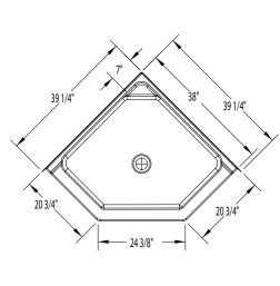
FEATURES | Ibs (kg) Dimensional Tolerance ± %". Dimensions needed for site preparation should be measured from the unit. Aquatic assumes no responsibility for preparatory work.
