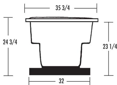
**FEATURES** lbs (kg) Dimensional Tolerance ± 3/8". Dimensions needed for site preparation should be measured from the unit. Aquatic assumes no responsibility for preparatory work.
