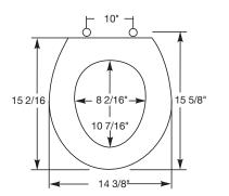
Seats shall be No. NW209E10 as manufactured by Church Seats. Seats shall be molded wood, multi-coat enamel finish to fit round American Standard Norwall toilet. Feature color matched bumpers and hinges with corrosion-free plastic nut and bolt. Color to be white.
