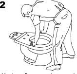
Unplug floor waste opening. Gently place the bowl, right side up, in position with the toilet mounting bolts protruding through the holes in the china base. Press down, with a slight twisting motion, on the top center, with your full weight. Make sure the bowl is as level as possible. If needed, you can use wedges under the bowl to help leveling. Put the washers (Marked: This Side Up) and nuts on the bolts. Tighten them evenly and snugly.
