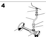
Connect the cold water line to the tank with your straight or angle stop. Place the washer, then the plastic nut on the tank end of the connecting pipe and bend the pipe to fit into the inlet hole on the water regulator. Tighten all coupling nuts securely. **DO NOT USE PLUMB-ERS PUTTY!**
