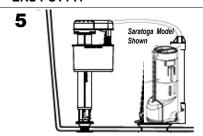
Connect the plastic tubing from the top of the water inlet regulator into its holding ring inside the overflow tube. If necessary, excess may be trimmed to eliminate any kinking of the line.
