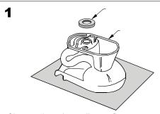
Clean the immediate floor area thoroughly. Insert new toilet bolts in the slotted flange, bolt heads down. The toilet bowl should be placed upside down, on soft material to prevent scratching. Place the slightly warmed wax ring in the circular recess in the base of the bowl.
