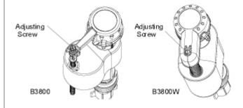
NOTE: The Pilot valve in this toilet is designed to operate at a minimum of 20psi and a maximum of 80psi. Turn on the water supply by opening the angle or straight stop. For proper flushing the tank Must fill to the Water Line marked on the inside of the tank. If the water is Below the Water Line mark, turn the screw clockwise, and if the water level is Above the Water Line mark, turn the screw counterclockwise.
