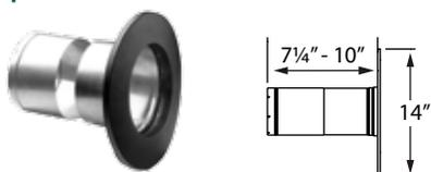
Use to penetrate masonry chimney to allow connection of DuraBlack or DVL to DuraLiner. Adapter must be used to attach the connector pipe to the masonry thimble.
