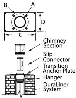
Use with Slip Connector and Hanger in chimney restoration to connect DuraLiner pipe to DuraTech, DuraPlus, or DuraPlus HTC Chimney. Painted black. Pricing for Transition Anchor Plates are listed under DuraTech, DuraPlus, and DuraPlus HTC.
