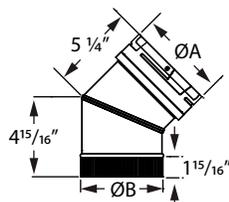
Use to offset obstructions as needed. Use as a insert connector to DuraLiner. Features built-in fittings for easy connection to DuraLiner. Elbows are single-wall.
