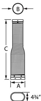
Use through damper and smoke shelf area. Use to connect from round stove outlet to oval DuraLiner. Use with DuraLiner Insulation Kit (ProMesh and ProFoil), where flex extends into clay liner, for zero clearance applications. Built from .016", 304 stainless steel, 4-ply construction.
