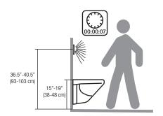
Installing highly reflective surfaces (such as mirrors) in the immediate vicinity of the water closet flush control should be avoided, as these can lead to incorrect releases and
