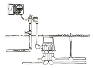
For high flow city water supplied installations using and in-line valve, ensure the HYDROTEK® Valve is installed as close to the in-line valve as possible. The 6000 Series Valve may be mounted below ground in a valve box (do not direct bury). Ensure backflow prevention is in compliance with local codes.
