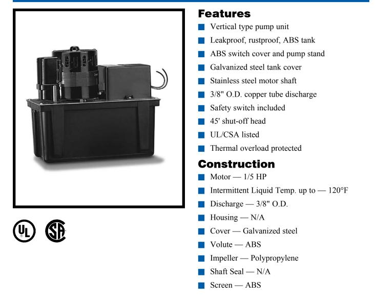
Large, 1 gallon, ABS plastic tank condensate unit. Pumps feature a vertical-type pump with stainless steel motor shaft and galvanized steel tank cover. Discharge is a 3/8" O.D. copper tube. Pump features a safety switch that can be connected to shut down the air conditioner condenser or wired to an alarm to warn of possible tank overflow. Pump is rated for high-efficiency gas furnace applications that produce an acidic condensate. Thermally protected motor is UL and CSA listed.
