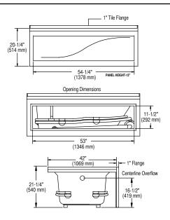
Unit is standard with removable access panels. Pump locations are shown for clarity. STD - standard pump location
