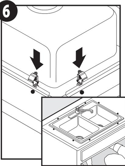
On underside of sink, attach installation clips by aligning clip to corresponding cutout in the integrated rails.
