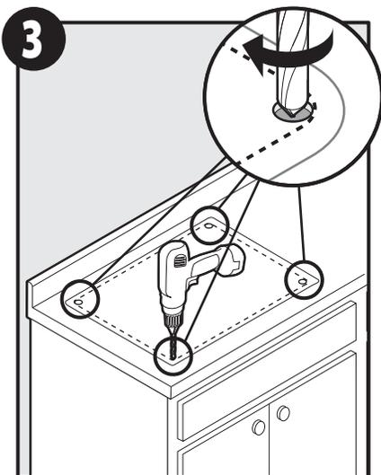
Drill pilot holes on cut line.
