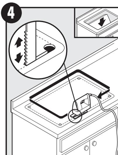
Carefully cut counter hole following inside of the cut line. Remove counter material.
