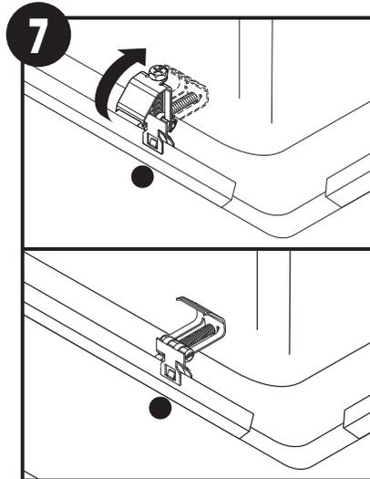
Center brackets along each side. 8 brackets are recommended. Once brackets are securely attached, swing them back toward sink bowl in preparation for installing sink into counter opening.
