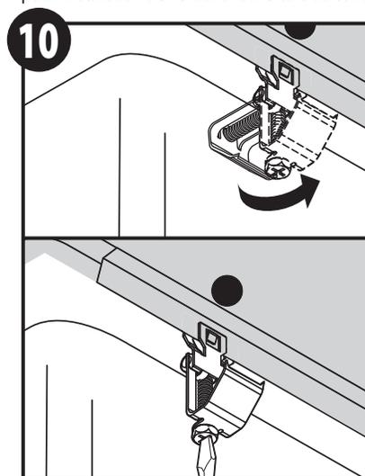
Once sink is located correctly in counter top, swing installation clips back down, so teeth are upward to grip underside of counter top, and tighten screws. It is only necessary to draw the rim down snugly to the counter top. Do not over tighten.
