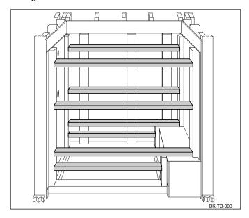
4. Insert small blocks between the front to rear panel braces and the back panel braces. These will apply pressure to the back panel to hold it in place.
