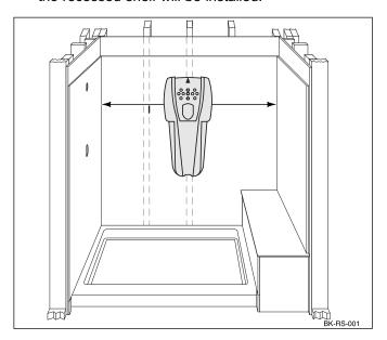
2. Mark the wall panel with the stud locations, as shown. A standard height for the recessed shelf would be 43" from the shower floor to the bottom of the opening.
