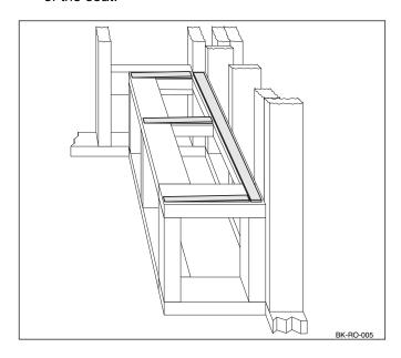
6. Determine the location of the shower base drain. Measure and cut a 6" opening for the drain in the subfloor.
