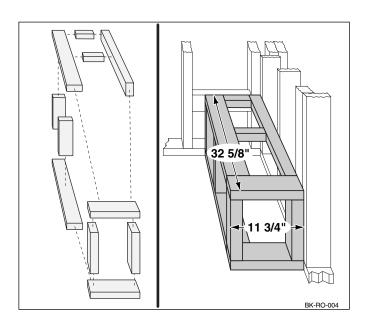
5. In order to eliminate standing water on the bench seat, cut and place three, 2" wide shims on top of each 2 x 4, as shown. Standard shim stock works well for these shims. The shims should be 1/8" thick and taper down to nothing. Also, place a 1/8" thick shim along the wall to completely support the back of the seat.
