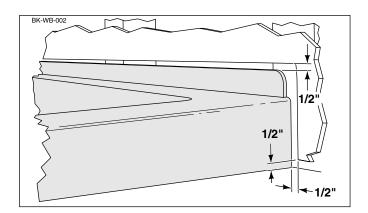
Apply a coat of water or oil-based primer/sealer to all the surfaces of the cement board or greenboard (follow the manufacturers' instructions). Allow the primer to dry thoroughly before applying any silicone.
