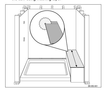
NOTE: The length of the seat can vary, depending on the amount of desired overhang and the type of material used to cover the end of the bench seat. The width of the bench seat is precut to 12-3/4" to provide a 1/2" overhang.
