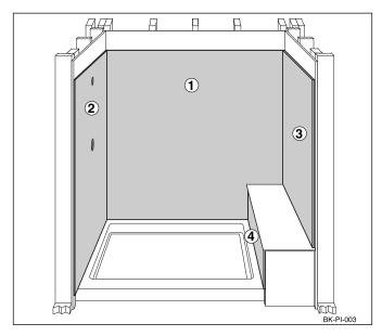
NOTE: When using an industrial grade hot melt glue gun in place of bracing, apply the silicone as stated in Step 2. Apply the hot melt glue to the panel, as needed, and press the panel firmly into place. The hot melt glue will hold the panel until the silicone bonds to the wall. This process is not recommended for the do-it-yourself homeowner.
