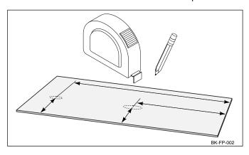
Cut clearance holes using a router, sabre saw, or hole saw. Drill from the finished side of the panel.
