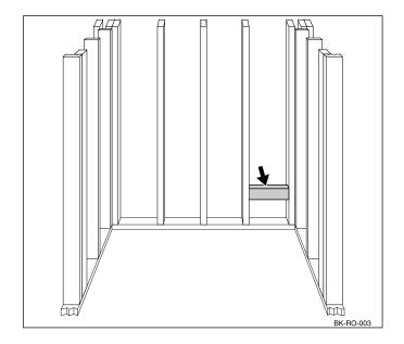
4. Construct the bench seat framework using 2 x 4 wood or steel studs. The framework for the seat must be 32-5/8" wide and 11-3/4" deep. The finished dimension of this seat, including the cement board, must be 12-1/4 x 33-1/8". Construct the framework, as shown.
