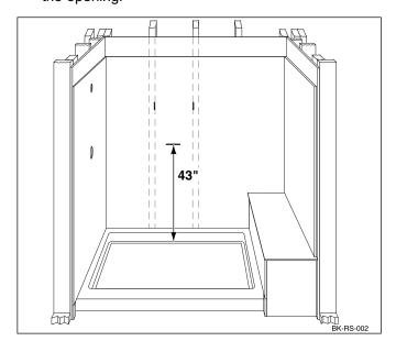
3. Mark the measurements, as shown, for the cut out onto the wall panel. Try to center the opening in the stud pocket. The wall stud opening shown is 16" on center, which creates a 14-1/2" opening.
