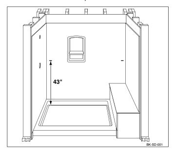
2. After marking the height, draw a 4" level-line on both walls. These lines will be used to align the top edges of the soap dish.
