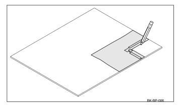
9. Remove the template(s) and place pieces of masking tape over the area where the saw contacts the Swanstone panel.
