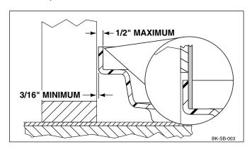
NOTE: The ideal placement of the shower base would be 1/2" from the inside lip of the shower base to the face of the stud. This dimension would allow the Swanstone wall panels to rest against the lip of the shower base once the moisture-resistant cement board is installed, as shown.
