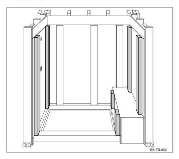
3. Install (wedge) four horizontal braces (eight total) against the side wall braces.
