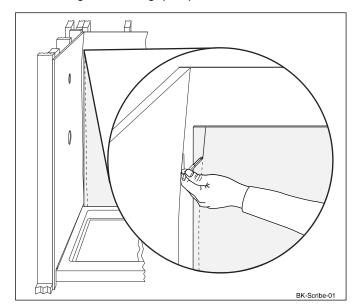
8. Place the back wall panel, finished side facing up, on a flat surface. Place the template(s) over the wall panel and carefully trace the outline of the template(s).
