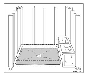
Place the shower base into the rough opening and firmly press it into the mortar/thinset. Make sure the side lips of the shower base are parallel with the wall with 3/16" gap between the face of the stud and the side lip.
