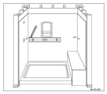
3. Dry fit the soap dish prior to applying silicone. If the wall is not exactly 90 degrees square, it will be necessary to sand one side in order to achieve proper fit. Use a course grit (60 grit) sandpaper.
