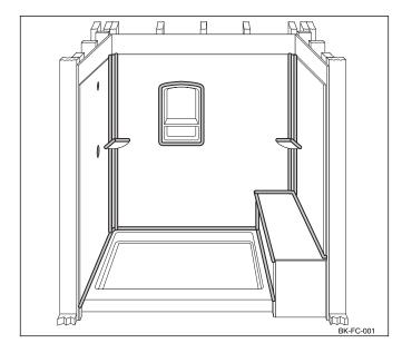
2. Apply white silicone sealant, as shown. This white silicone sealant is nonpaintable.
