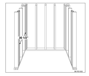
3. Add a 2 x 4 wall brace to attach the seat framing. The height of the brace should be the same height as the seat, which can vary according to personal needs.
