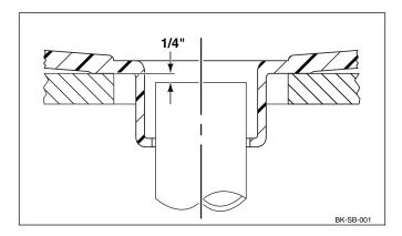
2. Remove the base and place up to 1/2" thick layer of mortar or thinset on the floor. This will ensure complete contact and support by the existing subfloor, eliminating shower floor flex during normal use. Taper the mortar/thinset to 1/4" thick around the floor drain. Mix enough material to cover an area approximately 1/2 x 24 x 42". Do not place the material closer than 2" to the edge of the shower base or the floor drain opening.
