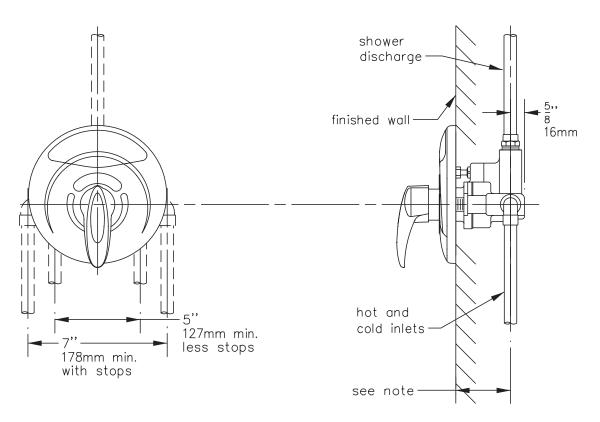
NOTE: 2-1/2" (64mm) min. 3" (76mm) max. On 2"x4" construction, use 2-1/2" (64mm) min. rough-in.
