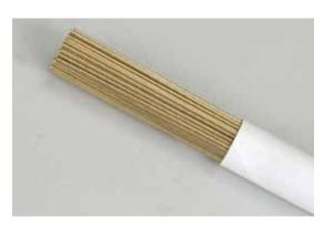
Bare brazing rod low furning highest quality. Balanced zinc and copper alloy. Excellent for brazing fenders, radiators, water tanks and sheet metal. 63,000 PSI tensile strength.
