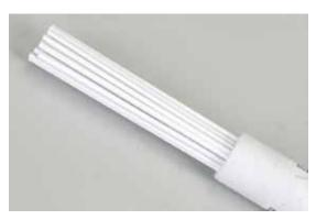
Flux coated, low fuming brazing rod. Provides all properties for best tensile strength and ductility. Rod fuses well with cast iron, malleable iron, galvanized iron, steel, brass and copper. 65,000 PSI tensile strength.
