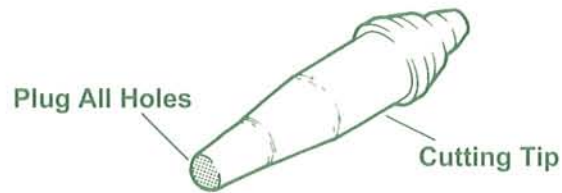
Figure 3: Plugged Cutting Tip for Leak Testing
