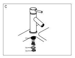
C. From under the sink, install the meatl wahser (14)and nuts (15) onto the mounting tube (13) Tighten the nuts to secure the faucet to the mounting surface.
