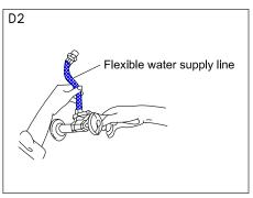
D2. Use Wrench to tighten the water supply hoses, please do not overtighten the connections.
