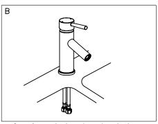
B. Place fange (11) and washer (12) under the new faucet. The faucet hole on the mounting surface should be 1 1/2" in diameter.
