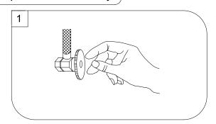
Shut off water supplies. Remove old faucet. Clean sink surface in preparation for new faucet.
