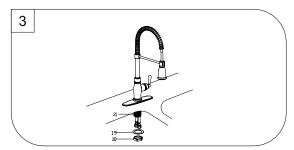
Screw the mounting stud into the body. Secure the faucet to sink by installing steel washer and nut onto it. Tighten with wrench.
