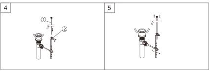
4. Insert lift rod (1) into sink hole, through the linker hole. Tighten the lock nut (2).
