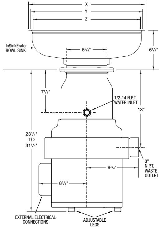
**IMPORTANT:** Use dimension chart below for adaptor height in place of ISE bowl sink height when mounting directly to a sink.
