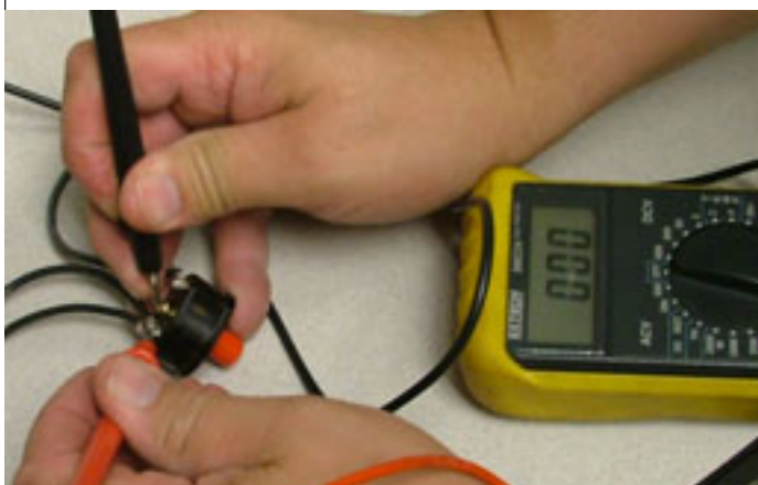
Figure 24. Testing Overload Protector
