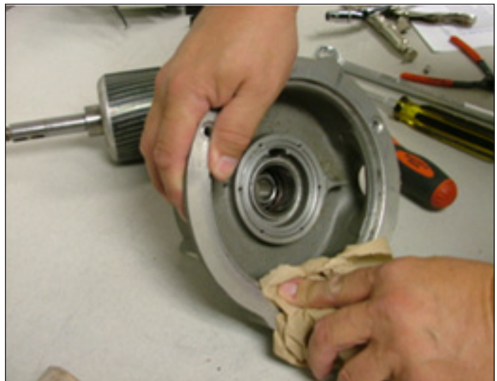
Figure 21. Cleaning Upper End Bell
