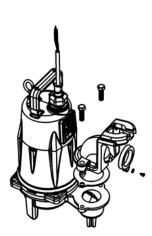
The GR22-LE and GR22-FL have a flanged claw that mounts directly to pump, They also have a 2" NPT threaded port for optional nipple connection.
