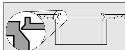
Knockout stays in one piece while it drops 1/8"—won't shatter into drain line.
