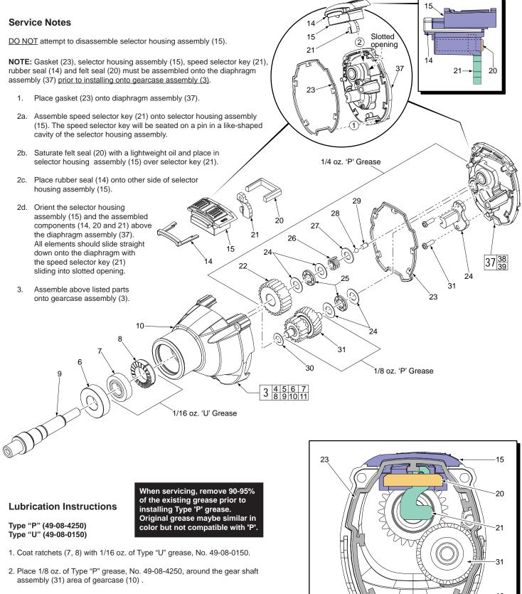
3. Lubricate gear assembly (parts 11, 22, 23, 24, 25, 26, 27, 28, 29, 30, 31, 35, 36, 38 and 39) using 1/4 oz. of Type "P" grease, No. 49-08-4250.
