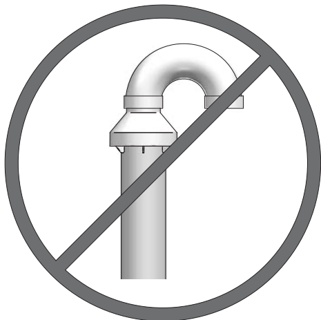
Figure 5-5 Do Not Install U-Bend to Rain Cap
