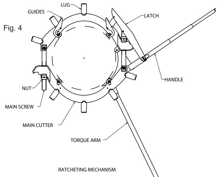
6. **Set-up for Ratcheting Mechanism**
