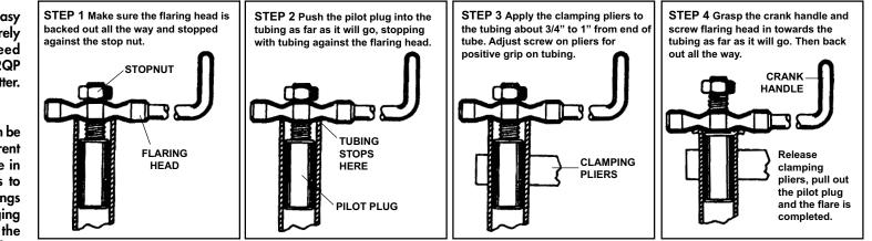
The diameter of the finished flare is determined by the amount of the flaring head between the stop nut and the meter. For smaller flare diameter, shorten the travel by screwing the stop nut down on the thread. To increase the flare diameter, screw the stop nut out further on the thread. Flare should be made slightly larger than the fitting threads so it "ripples" over the threads. Follow manufacturer's instructions for wrench tightening of fitting.
