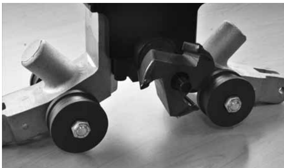
3. Tighten PVC Bevel Cutter onto Long Arbor
