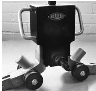
2. Tighten Long Arbor onto motor unit
