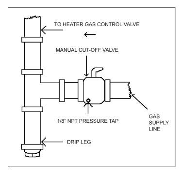
The appliance and its individual shutoff valve must be disconnected from the gas supply piping during any pressure testing of that system at test pressure in excess of ½ psig.
