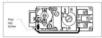
Fig. H-2: Pilot Flame Adjustment
