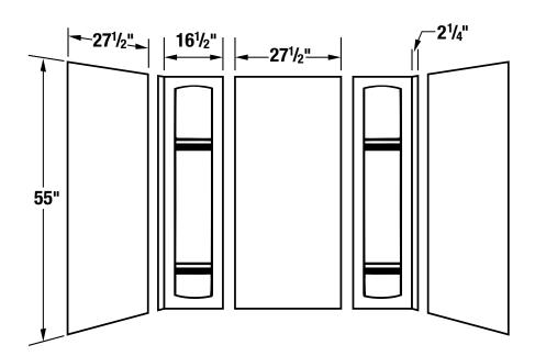
**General:** Furnish and install per plans, DURAWALL® Bathtub Walls model 950, as manufactured by E.L. Mustee & Sons, Inc. The white thermoplastic wall system shall be 5-piece construction with four built-in shelves and seamless, overlapping corner panels.
