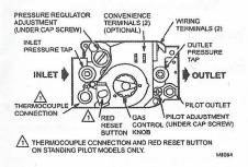
Fig. 1. Top view of VR8200 combination gas control.
