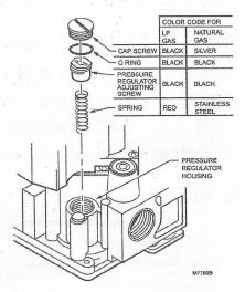
Fig. 2. Conversion kit installation in regulator.
