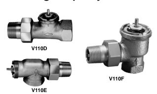
High Capacity Thermostatic Radiator Valves with T104 Thermostatic Actuators provide precise and automatic control of room temperature in two-pipe systems by modulating the flow of hot water or steam through free-standing radiators, convectors and other heating units with high capacity requirements.
