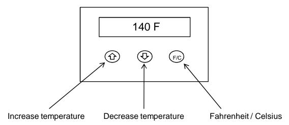
To trouble shoot the display board, shut off power to the unit. Press and hold all three buttons. While buttons are depressed, re-energize the unit. If display board is working properly, the word "Yes" will display. If the board has a fault it will display "No". Call technical support for a replacement.
