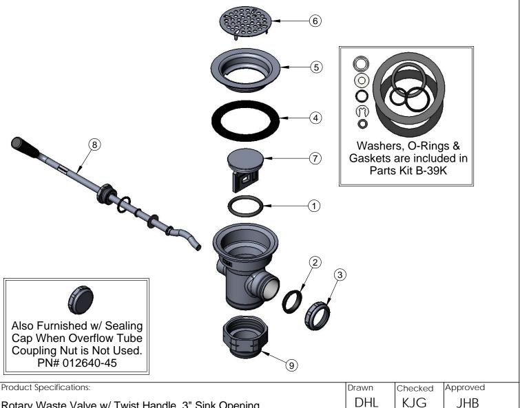
Rotary Waste Valve w/ Twist Handle, 3" Sink Opening, 2" NPT Male Outlet & 1 1/2" BSP Male Adapter
