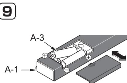
**11** Temporarily place the remote control in the position determined in **10** and confirm the signal reception of A-1.
