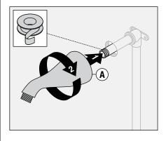
5) Install showerhead (B) to shower arm (A) turning clockwise to tighten.
