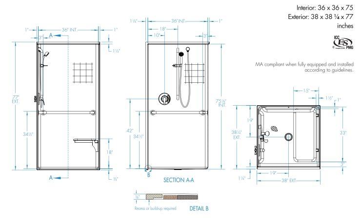
FEATURES Dimensional Tolerance ± %". Dimensions needed for site preparation should be measured from the unit. Aquatic assumes no responsibility for preparatory work.
