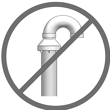
Figure 5-5 Do Not Install U-Bent to Rain Cap
