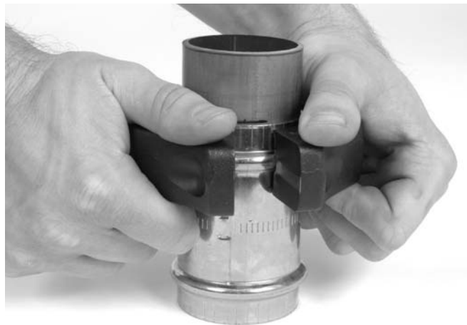
Figure 8 – Installing Press Ring Onto Fitting
