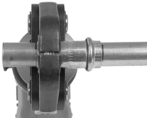
Figure 7 – RP 340 Tool Square To Tubing
