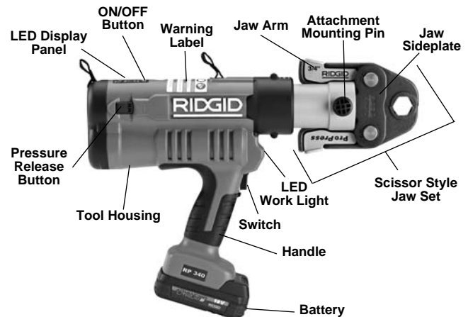
Figure 1 – RP 340 Press Tool and Jaw Set
