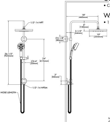
NOTE: 1. All dimensions are in inches (millimeters) unless otherwise specified and are subject to change without notice. 2. Waterslide bar supply nipple has  $\frac{1}{2}$  NPT male threads.
