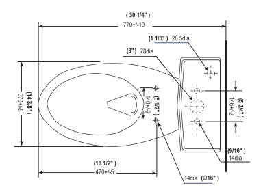
IMPORTANT: These dimensions are nominal and vary within the range of tolerances established by ASME standard A112.19.2.
