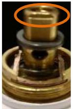
21. Reassemble the bearing washer into the Retainer Nut. The lip of the bearing washer goes into the Retainer Nut first. Then hand tighten the Retainer Nut back onto the faucet. Next, use pliers to tighten this an additional 1/8 of a turn.
