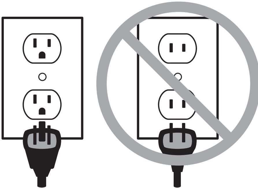
If repair or replacement of the cord or plug is necessary, do not connect the grounding wire to either flat blade terminals. The grounding wire is the insulation wire with a green surface that does or does not have stripes.
