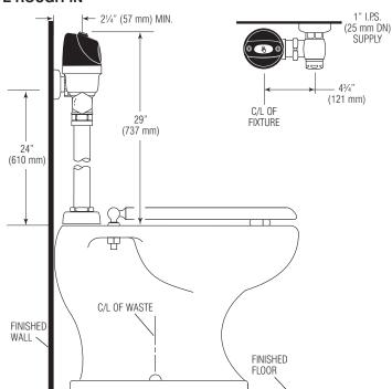
The Model 8115 valve is designed for installations where the water supply is roughed-in 24" (610 mm) above the top of the water closet. For new installations, Sloan strongly recommends the use of our Model 8111 which has a shorter installation height.
