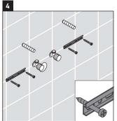
For wood stud walls, bolts should be screwed into wood backing.
