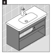
Slide the vanity under the washbasin. Tighten mounting bolts with a wrench until the washbasin is stable.
