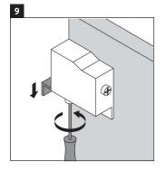
Using the crewdriver adjust the vanity mounting hinge system counter-clockwise.
