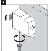
Using the screwdriver adjust the vanity mounting hinge system clockwise.
