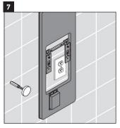
Lift the mirror backing up and onto the mounting brackets.
