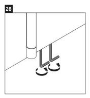
Using allen wrench, tighten the top middle screw clockwise one turn 90 degree or counter-clockwise one turn 90 degree until desired leveling of the hinged mirror has been reached.
